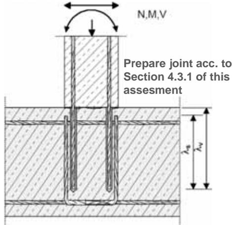
**Figure A3:** End anchoring of slabs or beams, designed as simply supported
