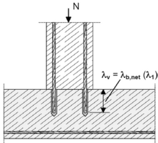
**Figure A5:** Anchoring of reinforcement to cover the line of acting tensile force
