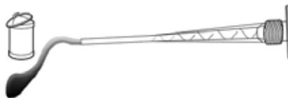
Extrude the first part of the cartridge to waste until an even colour has been achieved without streaking in the resin
