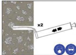
**If the hole collects water after the initial cleaning this water must be removed before injecting the resin.**
