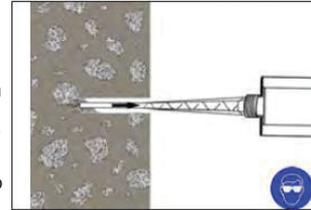
6. Insert the mixer nozzle (resin stopper / extension tube if applicable) to the bottom of the hole. Begin to extrude the resin and slowly withdraw the mixer nozzle from the hole ensuring that there are no air voids as the mixer nozzle is withdrawn. Fill the hole to approximately  $\frac{1}{2}$  to  $\frac{3}{4}$  full and remove the mixer nozzle completely.
