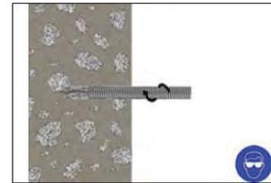
8. Any excess resin should be expelled from the hole evenly around the steel element showing that the hole is full. This excess resin should be removed from around the mouth of the hole before it sets.
