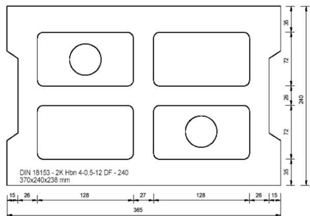
Concrete masonry unit Hbn 4-12DF
