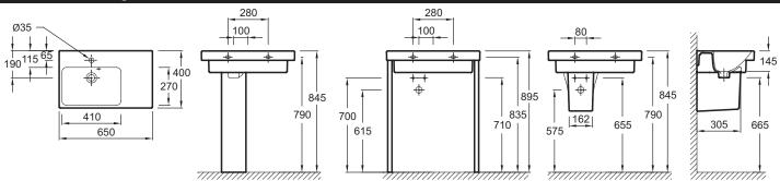
Product Specification: 1-hole vanity top 65 cm. 4946CK. Collection: REACH. Dimensions: 65 x 40. Weight: 19.8 kg. Material: Ceramic. Installation: Self-supporting.
