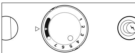
Press knob B fully in and hold it there; now press the piezoelectric igniter C. Check for a flame though hole A. Once the flame is on, continue holding knob B pressed in for a further 20 seconds or so. If the pilot flame does not stay on, repeat the above procedure.
