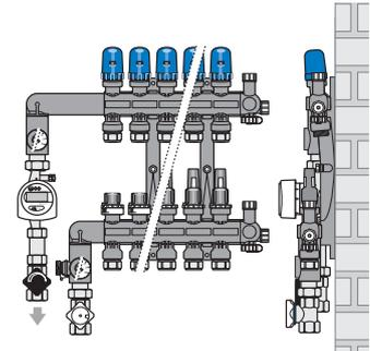
With heat meter - installed vertically
