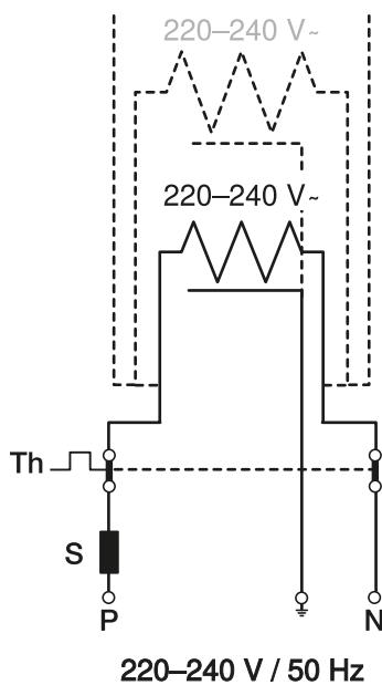
To switch off the heater during warmer seasons, use a thermostat with an outside temperature sensor.
