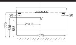
Product Specification: BASE unit 57.5 cm. EB1045. Collection: REPLAY. Dimensions: 57.5 x 45 x 47. Weight: 29 kg. Installation: Wall-hung with or without feet.
