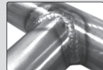
Fig. 6. Stainless steel tubes welded using the TIG method
