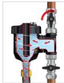
3. Open outlet and drain valves
